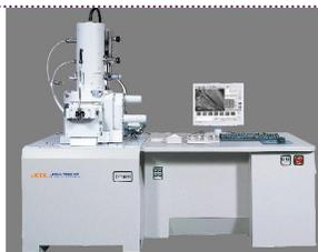
The [JSM-7001F](#) features a unique in lens field emission gun that delivers more than 200 nA of beam current to the sample. An extremely small probe diameter at low kV and high current is optimal for characterization of nanostructures with a resolution of 1.2nm at 30kV. The JSM-7001F is ideal
