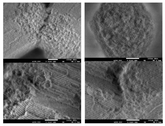
Sample: Mesoporous Silica which is: nonconductive, porous, has a poor SE yield, charges easily and has structures at the single digit nm scale. This type of sample needs to be imaged at high mag and ultra-low voltage to eliminate charging and edge effect. Conductive coating is not an option.
