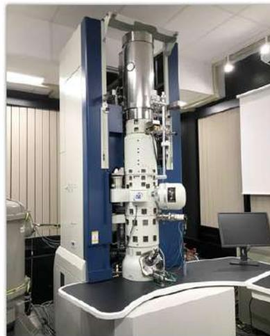
Groundbreaking TEM technology! A newly developed magnetic objective-lens system for a magnetic-field-free environment at the sample position enables direct, atom-resolved imaging of magnetic materials such as silicon steels. Developed by Prof. Naoya Shibata at the University of Tokyo and JEOL Ltd.
