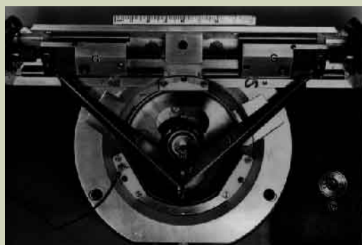
Fig.2. Laboratory-made universal 45° double-tilting stage viewed from the top. The specimen cartridge C shown separately is airlock-transferred to the cartridge holder H. It is tilted on moving the tongs T by means of gears G (G. Kästner, 1977).
