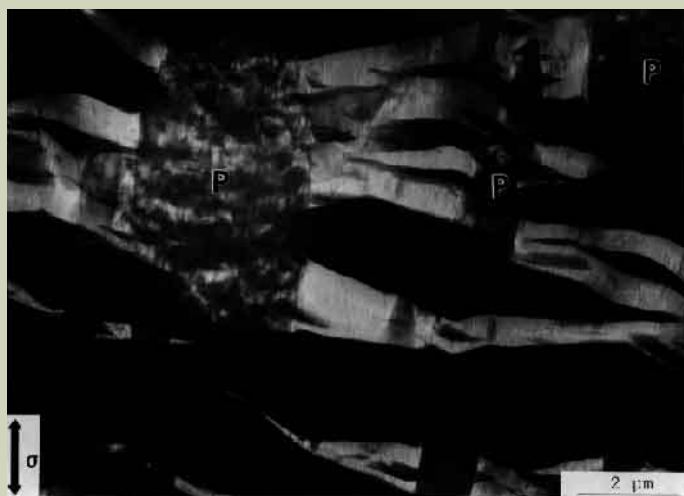
Fig.4. Thin section of high-impact polystyrene: Tensional strain (applied in vertical direction) is elongating the globular rubber particles P (of about 2\ \mu\text{m} in size) and opening crazes (bright, horizontal layers). Within each craze, fine fibrillae represent polystyrene heavily elongated by strain. Without the optimized fraction of rubber particles, the crazes would elongate catastrophically until the material breaks (G. Michler, 1976).
