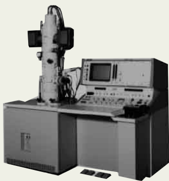
c. JSM-890 (first in-lens FESEM).
