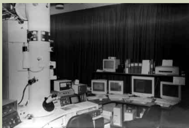
Fig.1. JEM-3000F analytical microscope at Oxford.
