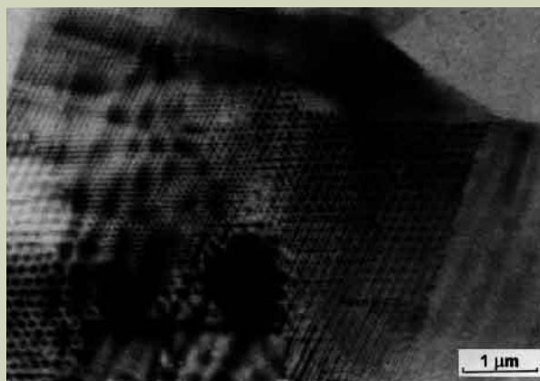
Fig.5. Liquid-crystal thin film prepared by vapour deposition onto a carbon film. The rod-shaped organic molecules of \text{C}_7\text{H}_{15}\text{O}-\text{C}_6\text{H}_4-\text{CH}=\text{N}-(\text{C}_6\text{H}_4)_2-\text{CN} are hexagonally packed within smectic layers of finite grain size. Overlapping layers give rise to Moiré patterns. Accelerating voltage 1000 kV (G. Kästner, Ch. Dietzsch, 1980).
