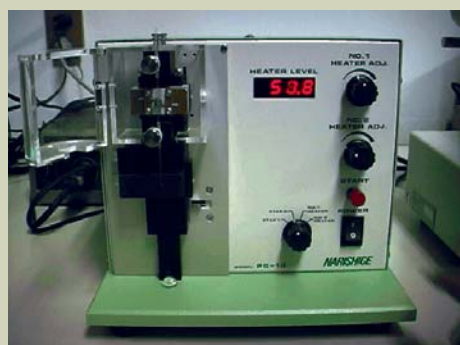
Fig. 1. Micro-pipette puller. Apparatus to make a probe by heating and cutting a glass rod.
