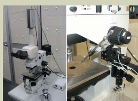
Fig. 3. Optical microscope with manipulator. Left: Overall picture of optical microscope with manipulator. Right: Enlarged picture of manipulator.
