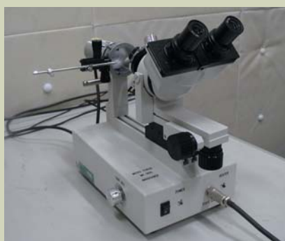
Fig. 2. Micro-forge. Apparatus for heating the probe tip and enlarging the surface area.
