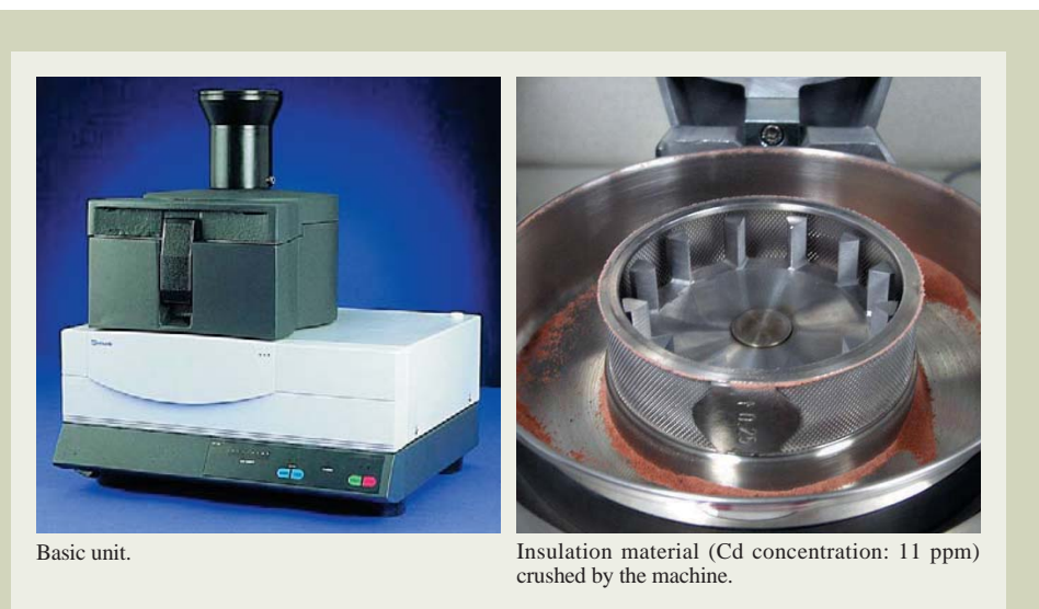
Fig. 4. Centrifugal crushing machine ZM100.
