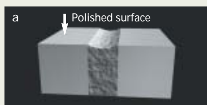
a) On material with different hardnesses, the polished surface becomes uneven as the soft portion is cut faster and easier.
