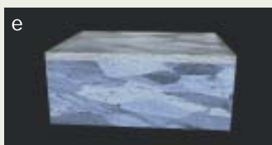
e) On metals, due to distortion caused by mechanical polishing on the polished surface, information about the crystal becomes difficult to obtain.
