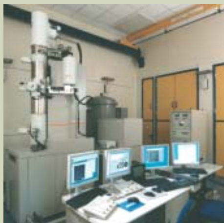
Fig. 1 The JEOL JEM-2200FS installed at Oxford showing major electron optical components and detectors. The local computer network controlling the microscope, correctors and ancillary devices is visible in the foreground.
