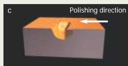
c) On soft material with a void, the material around the void stretches and deforms.
