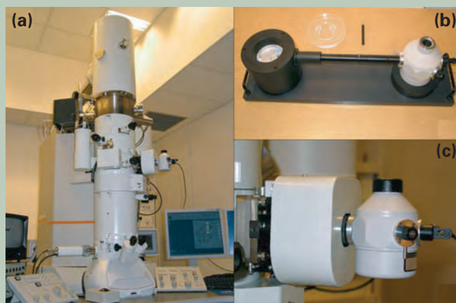
Fig. 2 Sample transfer to the electron microscope. (a) Side-entry Gatan 626 cryoholder inserted in goniometer of a JEOL JEM-2100F electron microscope. The sample stage of the microscope is nitrogen cooled (arrow), to prevent contamination. (b) cryo-transfer station, with cryoholder Gatan 626 inserted in the transfer chamber. Such device allows the positioning of the grid on the tip of the cryoholder under liquid nitrogen. The Dewar of the cryoholder is also filled with liquid nitrogen to maintain the sample cooled, even during the insertion of the cryoholder in the electron microscope. (c) Close view of the cryoholder once inserted into the electron microscope.
