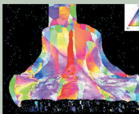
Fig. 2 Channeling images of electrode plating (FIB).
