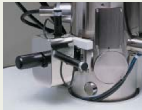
Side-entry goniometer stage
