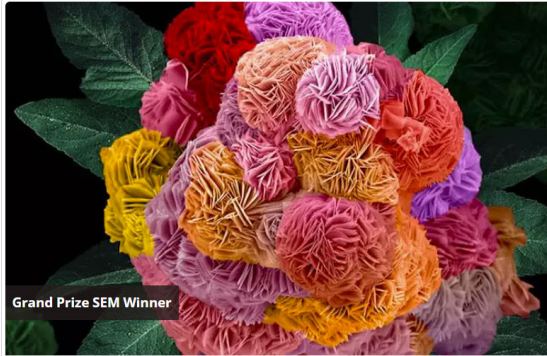
Grand Prize SEM Winner TITLE: Flower power; SUBJECT: Vanadium oxide nano structure synthesized from two-dimensional vanadium carbide MXenes; CREDIT: Yeonjin Baek, Auburn University; METHOD/INSTRUMENT: JEOL JSM-7000F SEM
