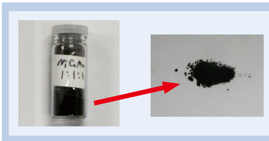
Fig. 14 NMC specimen for Li-ion battery actually used in our experiment (Mn, Co and Ni = 1:1:1).
