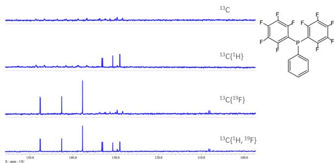
**Figure 9.** Another example of the amazing improvement obtained by  $\{^1\text{H}, ^{19}\text{F}\}$  for  $^{13}\text{C}$  observe with a fluorine containing molecule.
