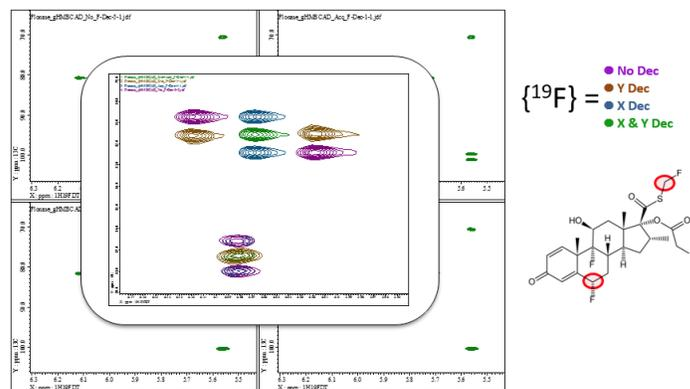
**Figure 12.** gHMBCAD example illustrating the simplifying effects of  $^{19}\text{F}$  decoupling for 2D  $^1\text{H}/^{13}\text{C}$  responses being applied in either, F1 (blue), F2 (brown), or both in dimensions (green). The diagonal purple responses clearly show how the  $^{19}\text{F}$  coupling exists in both dimensions.
