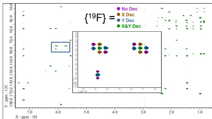
**$^1\text{H}$ - $^{13}\text{C}$  gHMBCAD,  $^{19}\text{F}$  Decoupling Simplifies Assignments, 25% NUS, 8 Scans 10mg Fluticasone Propionate/DMSO- $d_6$ .**
