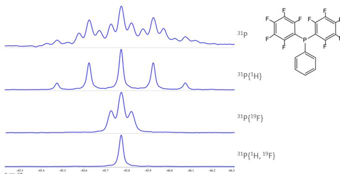
**Figure 10.** Effects of all combinations of  $^1\text{H}$  and  $^{19}\text{F}$  decoupling for a  $^{31}\text{P}$  resonance. In this figure the results for either no decoupling or single nucleus decoupling have the vertical scaling greatly increased relative to the  $\{^1\text{H}, ^{19}\text{F}\}$  example.
