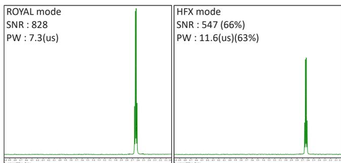
Figure 2.  $^1\text{H}$  signal to noise and  $pw90$  for a 500 MHz ROYAL-HFX Probe in single and dual-tune illustrating the expected changes in performance when switching modes.
