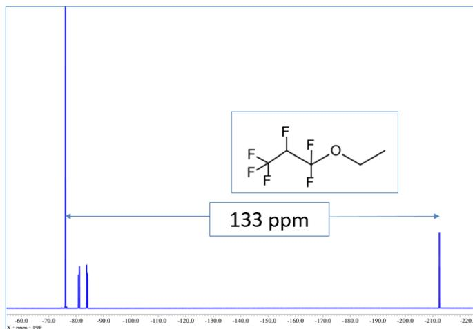
Figure 5.  $^{19}\text{F}\{^1\text{H}\}$  1D spectrum for a fluoro-ether illustrating the potential for large  $^{19}\text{F}$  frequency bandwidth.
