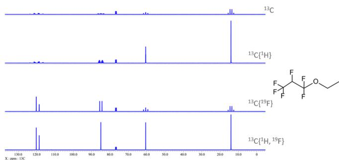
**Figure 8.** Full  $^{13}\text{C}$  spectrum for the fluoro-ether example showing all possible combinations of  $^1\text{H}$  and  $^{19}\text{F}$  decoupling. Results are shown with identical scaling to accentuate the dramatic improvement to  $^{13}\text{C}$  spectra of fluorine containing molecules by dual  $\{^1\text{H}, ^{19}\text{F}\}$ .
