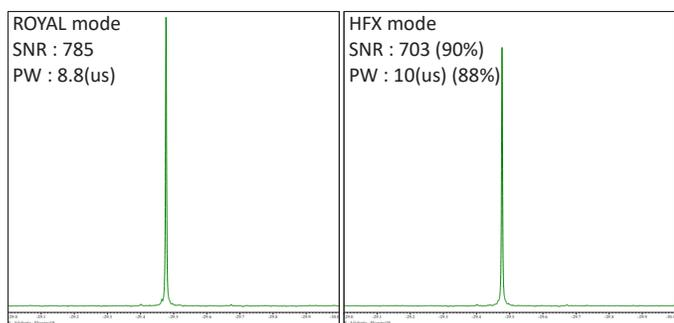
Figure 3.  $^{19}\text{F}$  signal to noise and  $pw90$  for a 500 MHz ROYAL-HFX Probe in single and dual-tune modes.
