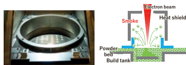
Fig. 5 Powder dispersal prevention "e-Shield".
