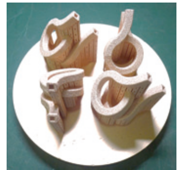
Fig. 9 Prototype Pure Copper Components: Heat Sinks.
