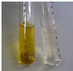
Fig. 1 RP oil (left: used, right: new)
