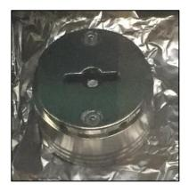
The sample holder (w/cap) is then removed from the glovebox and transferred into the load lock of the SEM. After the airlock is evacuated, the user can open the cap and put the sample into the FE-SEM without air exposure.
